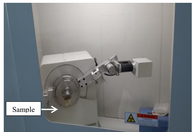
Figure 6. The specimen inside the X-ray diffractometer
