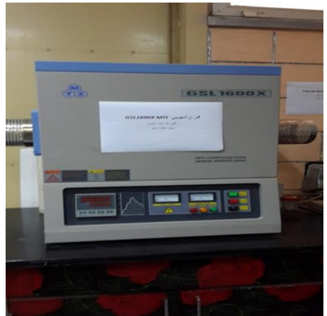
Figure 5. The vacuumed furnace
