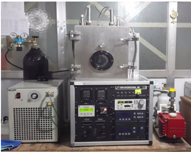
Figure 3. R.F. Magnetron sputtering technique system
