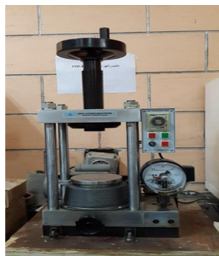
Figure 2. The electrical hydraulic press
