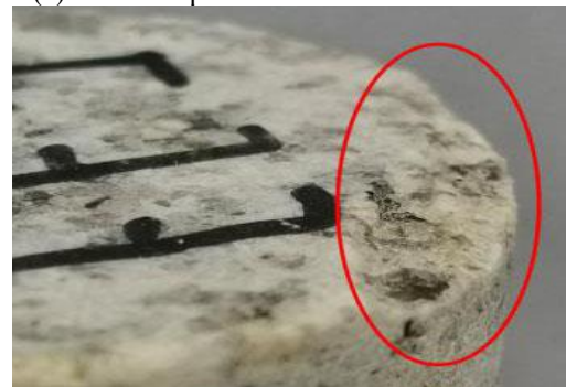
(b) Rock debris peeled off after freeze-thaw cycles
