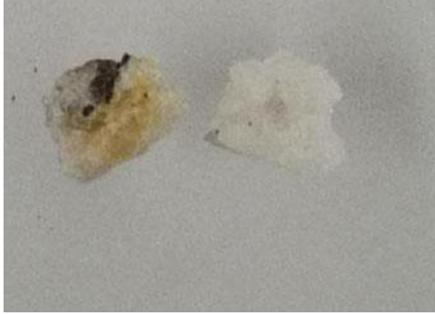
(d) Rock particles fallen off from the sample under freeze-thaw effect
