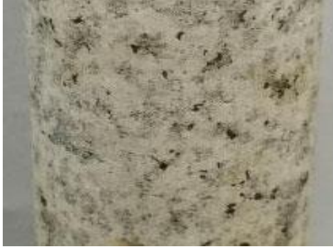
(c) Rock debris peeled off from the sample under freeze-thaw effect
