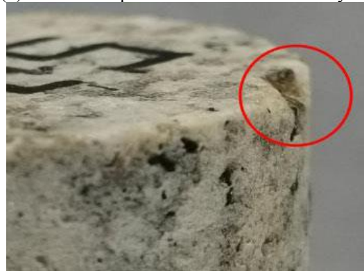
(c) Rock particles fell off after freeze-thaw cycles
