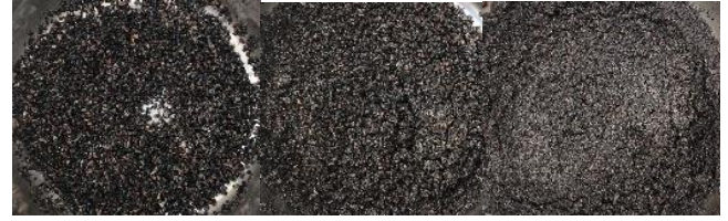
Figure 1. Filtered oil shale wastes of three different particle sizes after soaked in diesel
