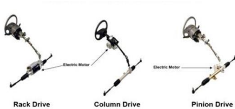
Figure 1. The steering systems with rack and pinion gear [1]
