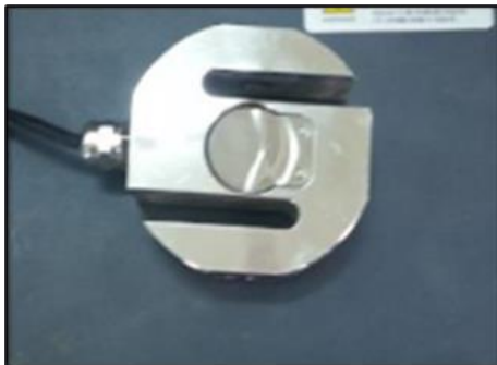
Figure 4. The compression load cell used in the study
