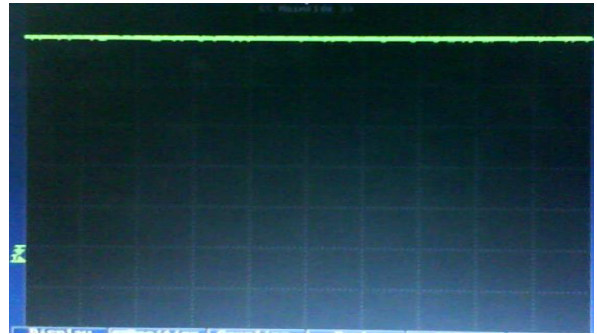
Figure 5.8 DC supply applied to Inverter Bridge
