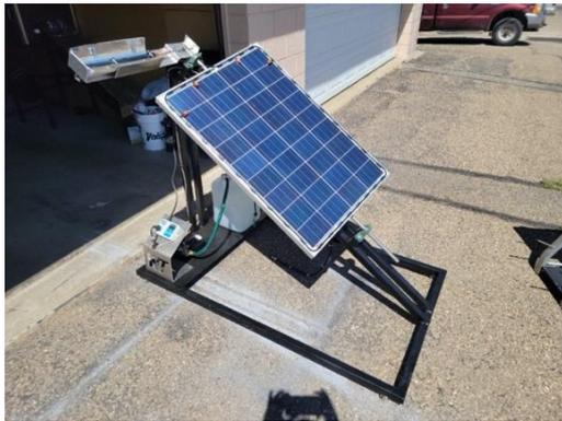
Figure 2. Overall setup of the solar tracking system
