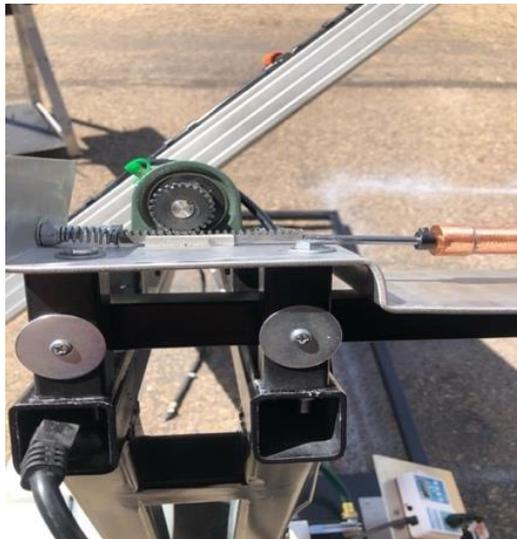
Figure 3. Rack and pinion gear system
