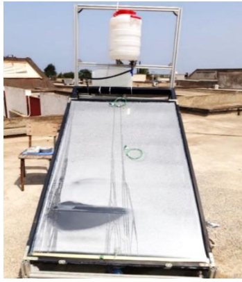
Figure 3. Experimental set up of novel cascade solar still
