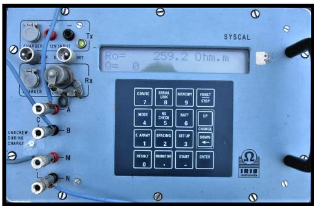
Figure 5. The standard resistivity meter model IRIS from IRIS Instruments France
