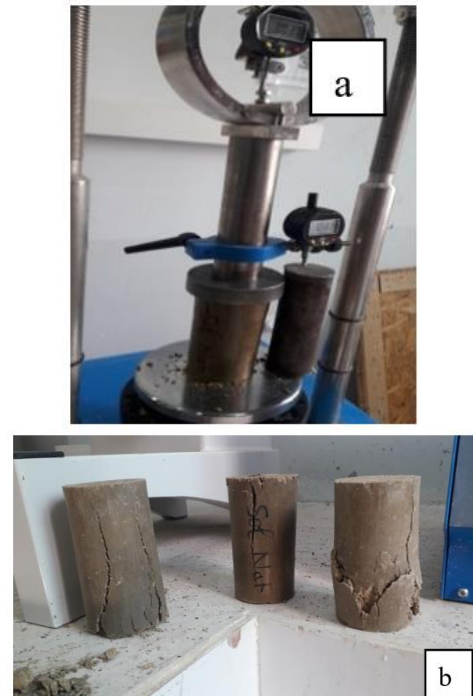
Figure 4. Typical failure of specimens after UCS test
