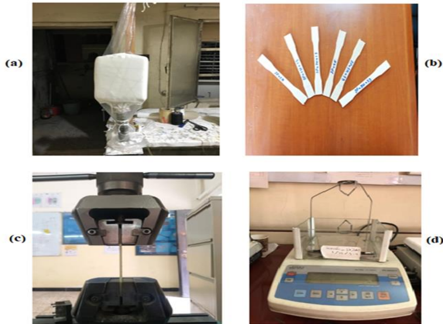
Figure 4. Experimental process: (a) Vacuum bag process, (b) Tensile test specimens, (c) Tensile test process, and (d) Density tester
