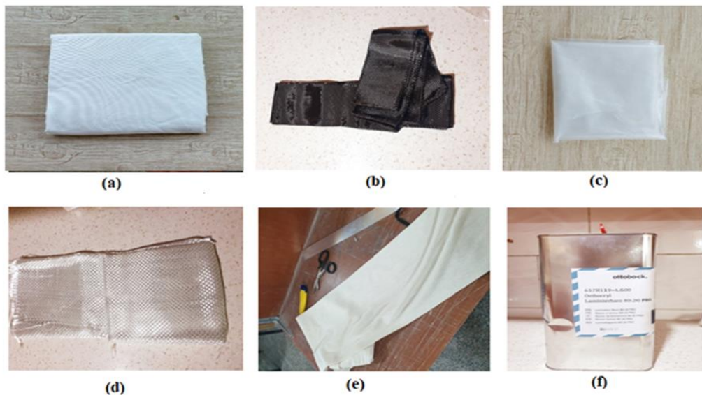
Figure 3. Materials employed in the current study: (a) UHMWPE woven fabrics, (b) Woven carbon fiber, (c) Polyvinyl alcohol (PVA), (d) Woven glass fiber, (e) Woven Perlon fibers, and (f) Epoxy resin orthocryl lamination
