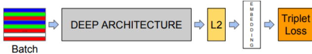
Figure 2. Structure of FaceNet model consisting of batch input layer, deep CNN architecture and L 2 normalization resulting in the face embedding [9]
