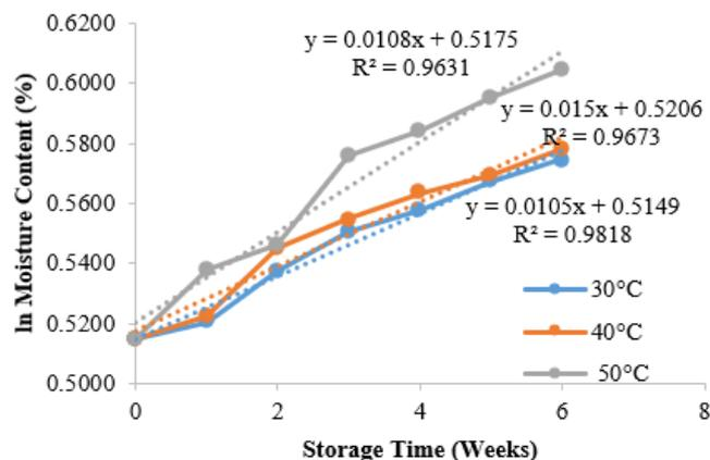
**Figure 2.** Order 1 linear regression of water content in instant chocolate vacuum packaged using PP plastic
