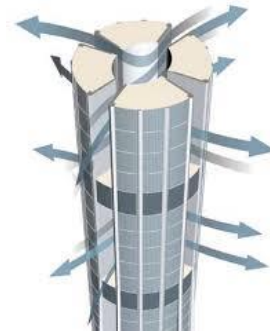
Figure 5. Two vertical slots of Nakheel Tower [19]
