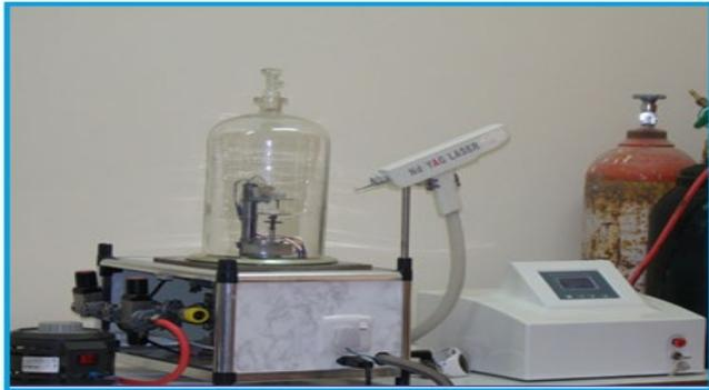
**Figure 2.** Experimental setup of PLD.
