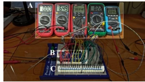
Figure 3. Photo of laboratory installation (A – block of control and measuring devices, B – tested microprocessor platform, C – block of loading of port groups)
