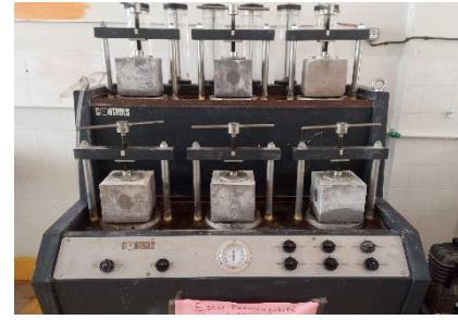
Figure 2. Apparatus for measuring water permeability (Water penetration depth)
