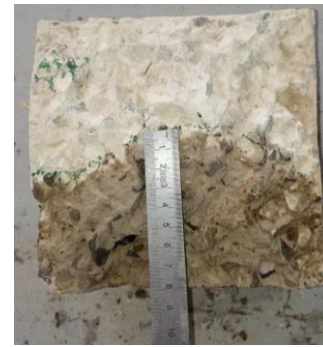
Figure 3. Penetration depth in concrete samples
