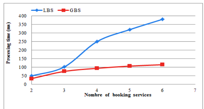
Figure 6. Effect of the number of services on the processing time for local and global booking skylines
