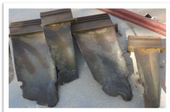
Figure 1. Corrosion in turbine blades
