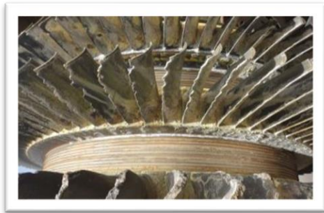
Figure 2. Hot corrosion attack to turbine blade
