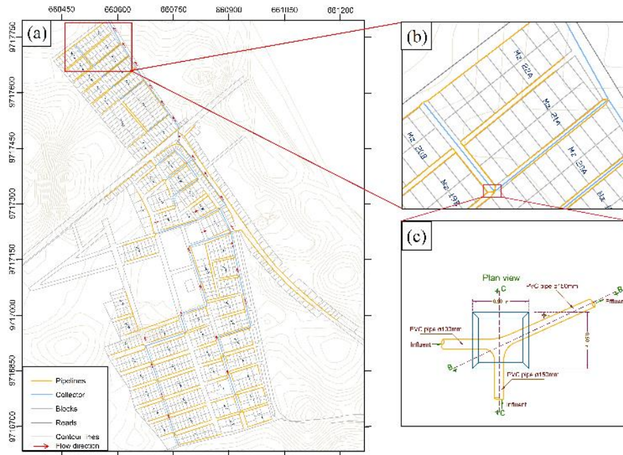
Figure 6. Sewerage system: a) general implementation, b) detail of strands, straps and collector, and c) detail home corner box
