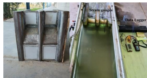
Figure 2. The model with data logger and strain gauge
