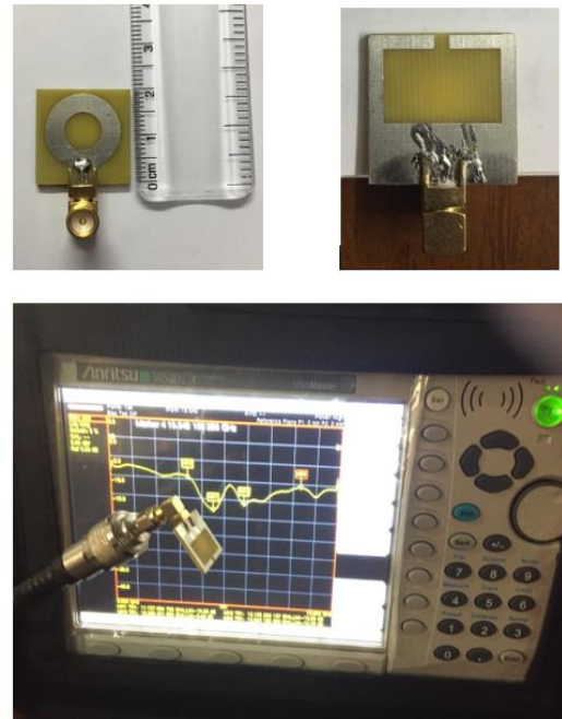
Figure 2. Photographic view of the proposed CSRR antenna and the Measurement set-up
