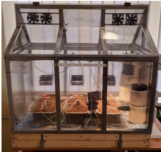
a) General view of the computerized greenhouse prototype (The dimensions of the implemented physical model of the greenhouse are the following: height–1.5m, length of base–1.5m, width of base–0.9m)
