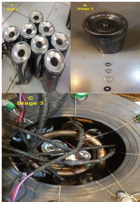
Figure 3. a) Injecting PCMs inside cylinders, b) Procedure of non-leakage packing for each cylinder, c) Insert the bottles in shell side of chamber to perform the test 1 and 2
