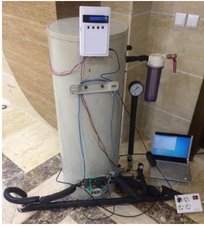
Figure 2. Latent Thermal Energy Storage System (TESS)
