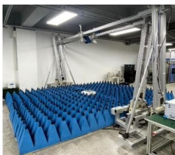
Figure 2. Test equipment for the arch method
