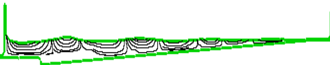
Figure 26. The streamline contour of first type of sandy coast bed in t=12
