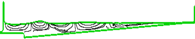
Figure 25. The streamline contour of first type of sandy coast bed in t=10
