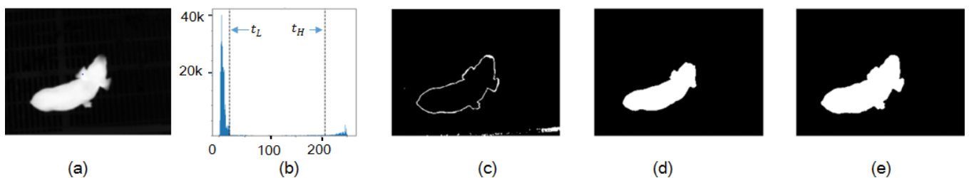
Figure 4. Graphical flow of the proposed image segmentation (a) Grayscale image (b) Selecting t_L and t_H from the histogram (c) Pixels labeled t_L (d) Pixels labeled by t_H (e) final segmentation result using the double thresholding method
