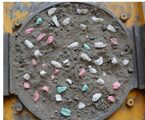
Figure 2. Distribution of blocks on the shear surface after the shearing was completed when the rock content was 40%
