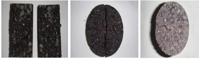
Figure 2. Failure forms of specimens
