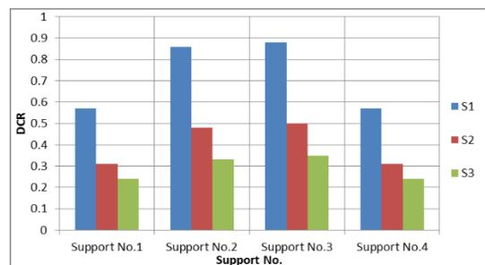
Figure 2. DCR in transverse direction of square form of pier
