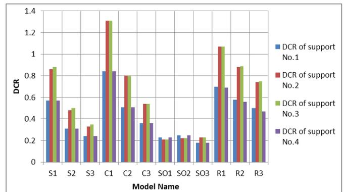
**Figure 18.** DCR in transverse direction of structural form of bridge piers
