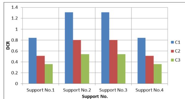
**Figure 4.** DCR in transverse direction of Circle form of pier
