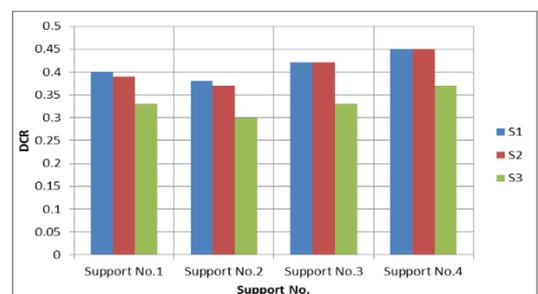
Figure 3. DCR in longitudinal direction of square form of pier
