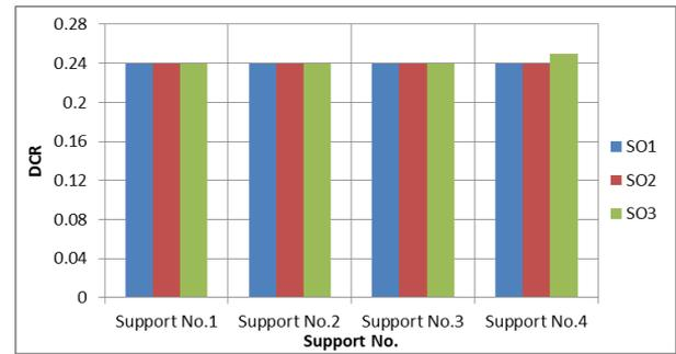
**Figure 6.** DCR in transverse direction of solid wall form of pier
