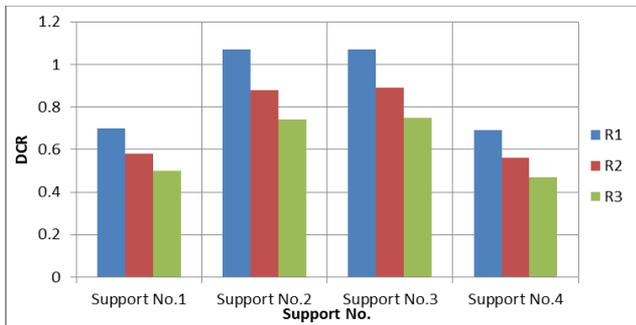
**Figure 8.** DCR in transverse direction of rectangular form of pier
