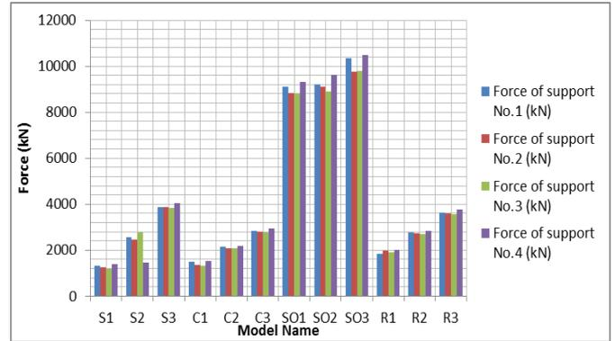
**Figure 16.** Force yielding points in longitudinal direction for bridges supports models
