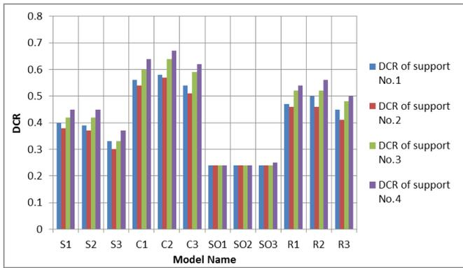
**Figure 19.** DCR in longitudinal direction of structural form of bridge piers
