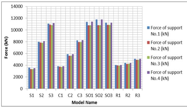
Figure 10. Force yielding points in transverse direction for bridges supports
