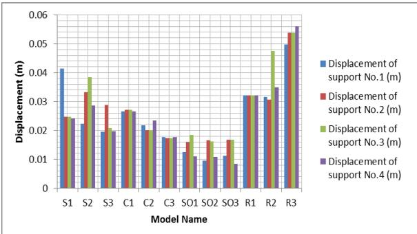
Figure 11. Displacement yielding points in transverse direction for bridges supports
