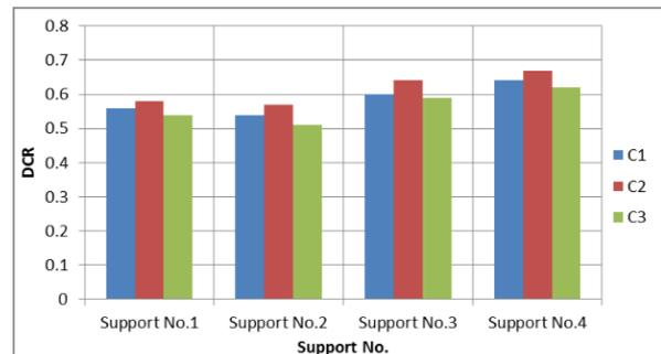
**Figure 5.** DCR in longitudinal direction of Circle form of pier
