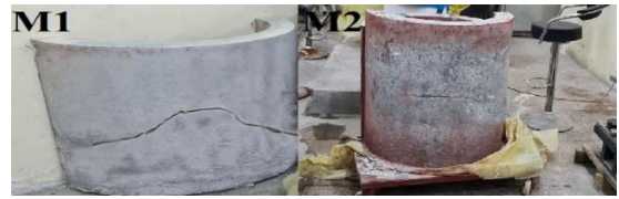
Figure 8. Deformation and crack propagation patterns
