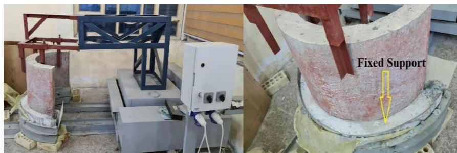
Figure 4. Concrete arch dam model with fixed support
