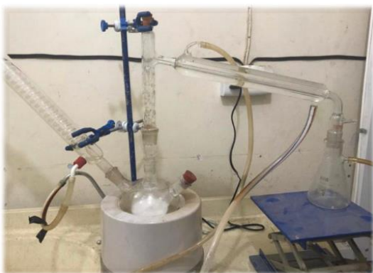
Figure 8. Method of converting DPET to fuel
