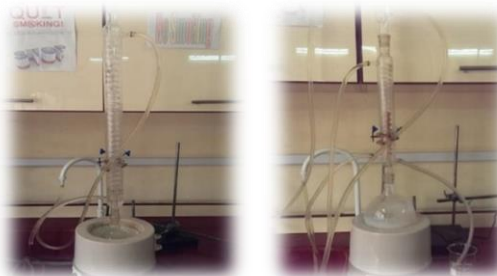
Figure 4. Close system of chemical recycling and after Separation of UN reacted EG. From mixture
