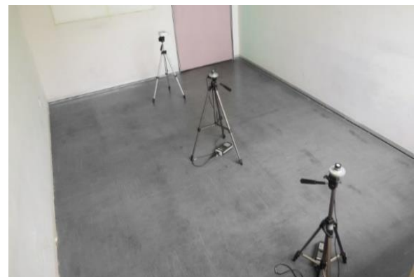
Figure 4. Geometry of the test room and locations of the illuminance meters for the field measurement
