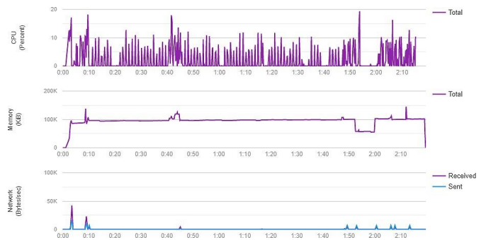
Figure 12. Driver Activity CPU, Network and Memory statistics for 2 min 19 sec
