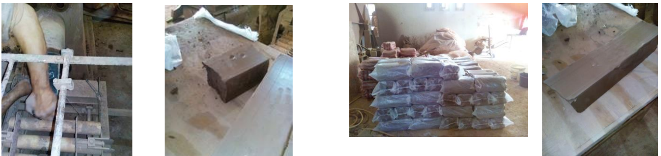
Figure 4. The blocks protected with plastic
