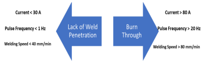
Figure 5. Cause and effect diagram of TIG welding parameters
