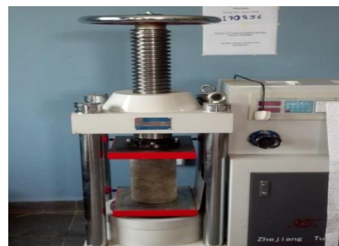
Figure 8. Compressive strength testing machine [14, 16]
