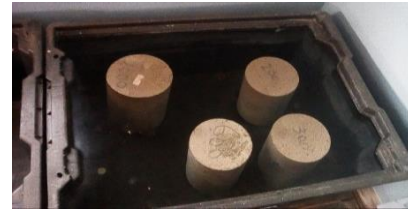
Figure 7. Immersion of concrete specimens for curing
