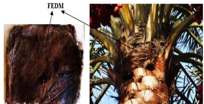
Figure 4. Palm fiber used as thermal insulation in the collector
