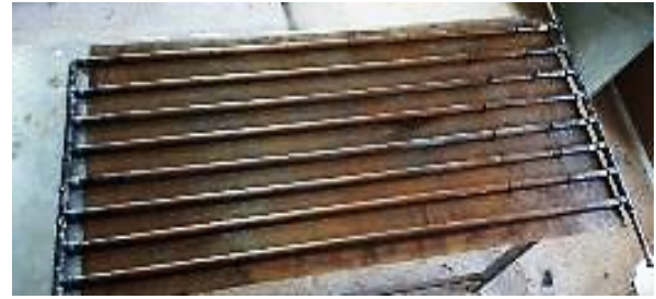
Figure 3. Copper tubes solar-collector (Image)
