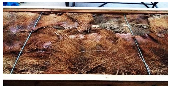
Figure 5. Palm fiber used as thermal insulator in the collector
