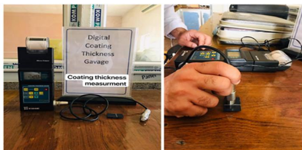
Figure 4. Thin-film thickness measurement (micro-printer)
