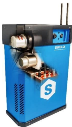
Figure 4. New compact set-up containing the DT5790, two detectors, the LiFePO 4 Battery and the Single Board Computer (SBC). Data are transmitted through Wi-Fi
