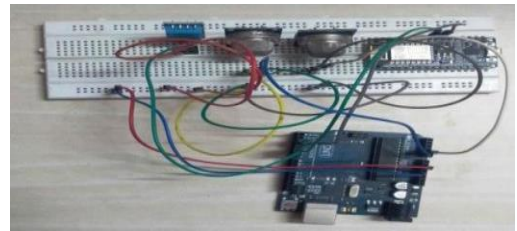
Figure 9. Arduino Configuration with the DHT11 / MQ2 / MQ135 Sensors
