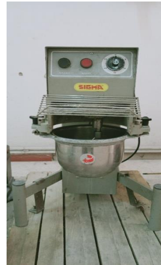
Figure 2. Picture of the mixer with a capacity of 5 kg
