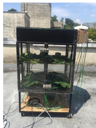
Figure 1. Photograph of greenhouse dryer consisting of solar collector attached to the drying chamber
