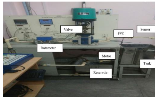
Figure 2. Experimental set up for liquid flow rate measurement
