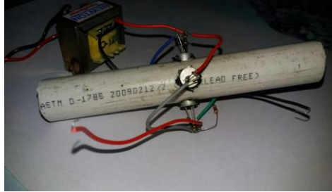
Figure 1. Semiconductor based Anemometer
