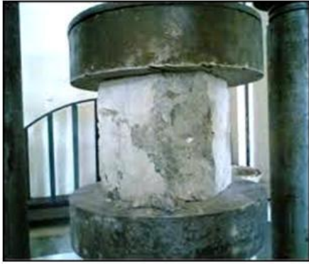
Figure 5. Experimentations for UTM Cube compressions test
