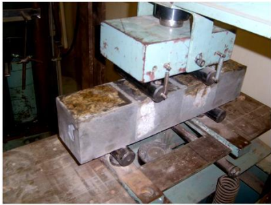
Figure 9. Flextural strength of concrete beam under considerations of load (unit flextural MPa=N/mm 2 )
