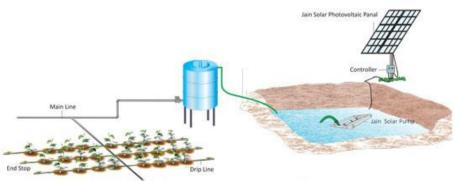
Schematic of Solar Powered Jain DripKit sourced through farm pond.
