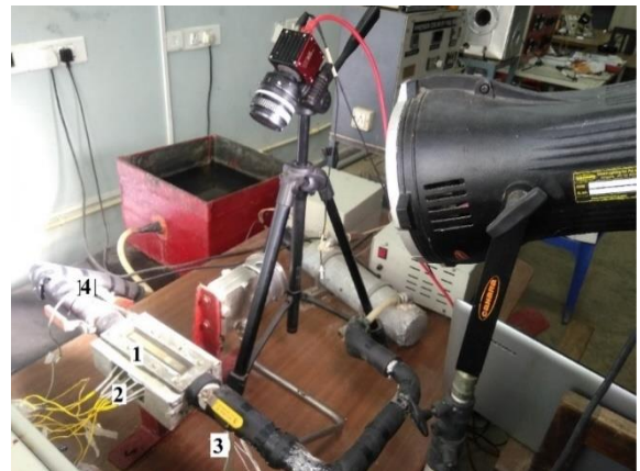
(1) Rectangular aluminum block consisting of two rectangular channels (2) Thermocouples to measure wall temperature (3) Thermocouple to measure channel inlet temperature (4) Thermocouple to measure outlet fluid temperature
