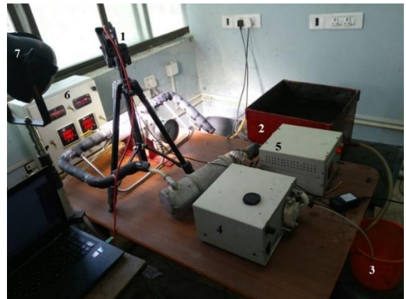
(1) High speed camera (2) Condenser coil dipped in ice water bath (3) Reservoir (4) Peristaltic pump (5) Preheater (6) Temperature indicator panel (7) Light source
