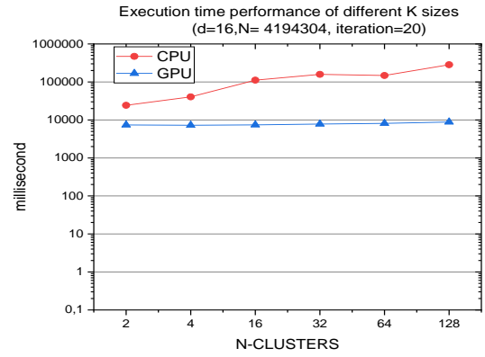
Figure 12. Execution time for k-means++ with varying cluster sizes on GPU and CPU when dataset=4194304
