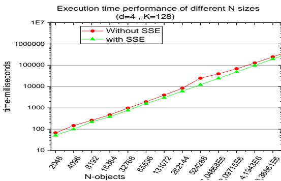
Figure 4. Execution time for the initialization step with and without using SSE instructions of k-means++ with varying object sizes when K-cluster =4
