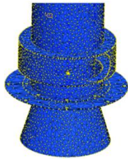
Figure 5. Close-up of discretized recuperative heat exchanger
