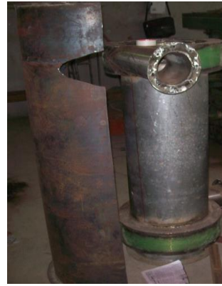
Plate 1: Recuperator outer casing & half covering drum
