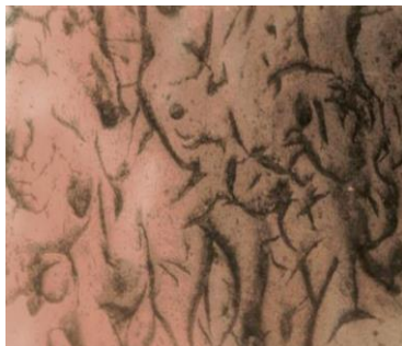
Figure 9. The white cast iron was largely grayed after high forming rates
